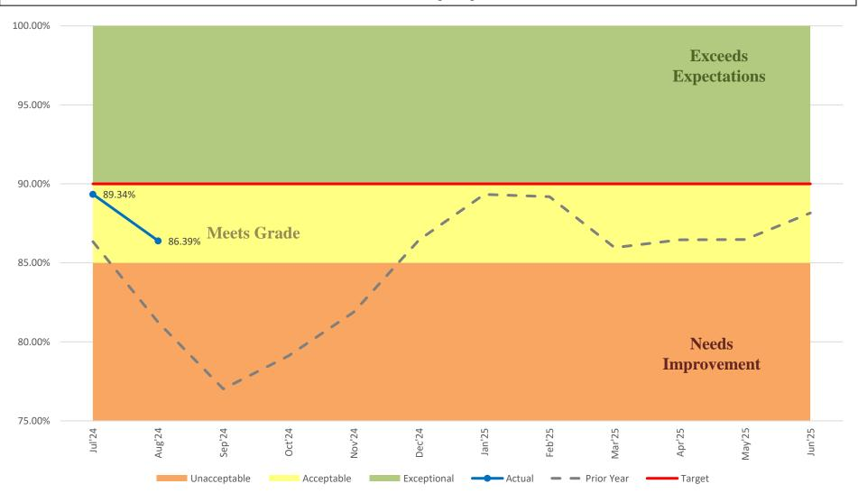
Mobility Mean Distance Between Failures measured as the average Mobility service miles between NTD reportable mechanical failures, i.e., those precluding a revenue vehicle from completing its revenue trip or starting its next scheduled revenue trip.
